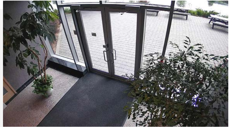
2.8mm lens. This wide-angle lens is very common in the industry, but you miss critical details due to the limited field of view.
